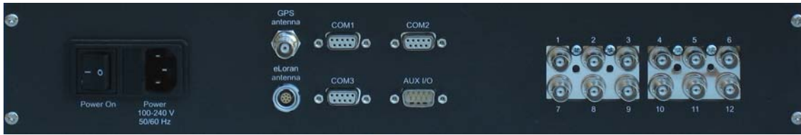
Figure 2-2 Picture of the interconnections on the rear of the UTC receiver
